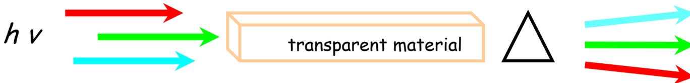
distinguishable photons in; distinguishable photons out, with little heat, no cross-talk, and a vast new set of architectures available. Variables include wavelength and polarization state.
